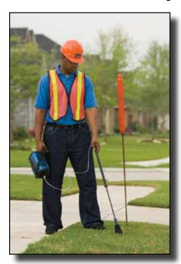
The **HEATH** Detecto Pak-Infrared (DP-IR<sup>™</sup>) is a highly advanced technology capable of detecting methane without false alarming on other gases. The DP-IR is the latest of a new generation of leak survey instruments from **HEATH** that will greatly improve the productivity and safety of a walking/mobile survey.
