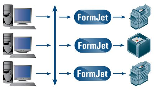
FormJet Pro arrives as a small powerful standalone device with your solution preinstalled. Just use the included network cable to connect the FormJet between your printer and network. No configuration required. The FormJet automatically adopts the printer's network configuration settings.
