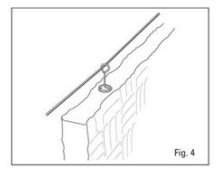
W4. Slip the eye loops over the cable (Figure 3). Turn the eye loops approximately ¼ turn counterclockwise so the eye loops are perpendicular to the baffle, locking the cable in place (Figure 4).
