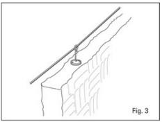
W2. Attach steel cable to one wall or I-beam with eyebolts and And turnbuckles.
