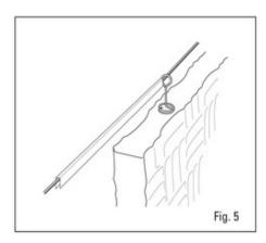
W6. Optional: Install a center support hook or eye in the middle of the ceiling to counter cable sag approximately 2 ½" over 80 feet. Slide baffles from each end of the cable to the center.
