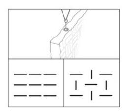
The baffles can be aligned in the same direction or arranged so that every other baffles is turned 90 degrees.
