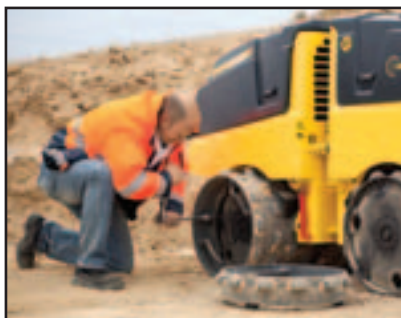
Easy installation of standard bolt-on drum extensions increases compactor versatility.
