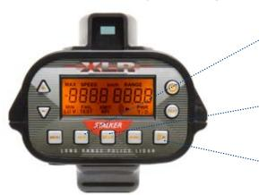
HUD Light switch - allows operator to increase or decrease with a single button the HUD intensity for proper viewing in all lighting conditions.
