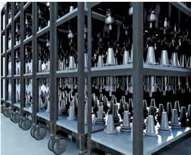
Machine tools can be fitted with RFID tags to track and download offset measurements (from presetter), set-up parameters, usage, and tool life data.
