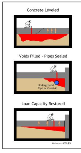
The URETEK Method is very effective in addressing these types of voids. The expansive, hydro-insensitive polymer material, which is at the core of the URETEK Method, drives out any standing water and aggressively fills voids. This also densifies the soil and prevents the expansion and formation of new voids in the future.
