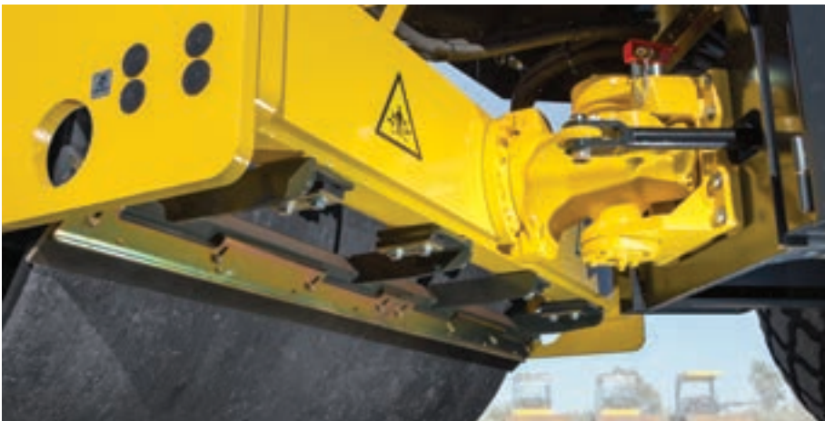
Maintenance free oscillating articulation joint.
