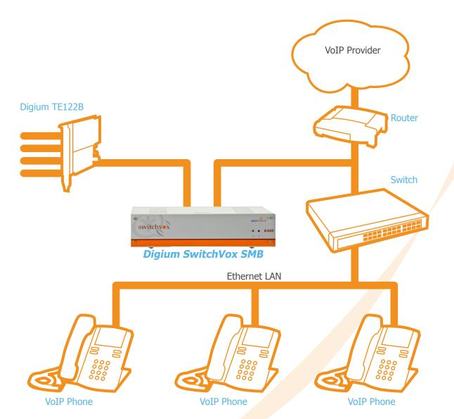
This set-up is different from your traditional PBX. Your traditional PBX uses its own closed network that interconnects your desktop telephones, PBX hardware and connection to the PSTN. The consolidation of networks that comes with using a VoIP Phone system is one of the benefits you will read about on page 7.
