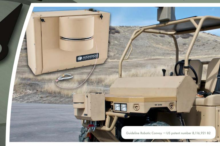
Guideline<sup>TM</sup> is a self-contained, robotic leader-follower kit which can be easily integrated with any existing robotic vehicle or appliqué kit. Through the use of a simple tether connection, the Guideline<sup>TM</sup>-equipped follower mimics the path of any leader with sufficient accuracy for lane-keeping at highway speeds.
