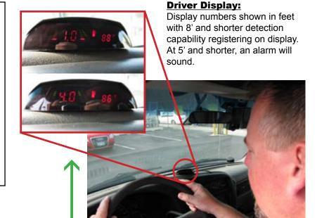
Wireless communication between control box & display unit shown above.
