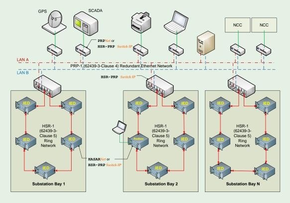
A simple HSR network consists of doubly attached bridging nodes, each having two ring ports, so nodes are restricted to be HSR-capable bridging nodes.
