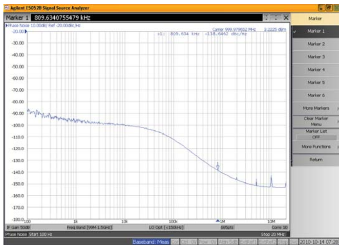
Fig. 1. Local Oscillator phase noise at 1 GHz (typical).
