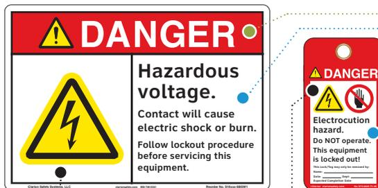
**Signal word** panels identify the hazard severity level.
