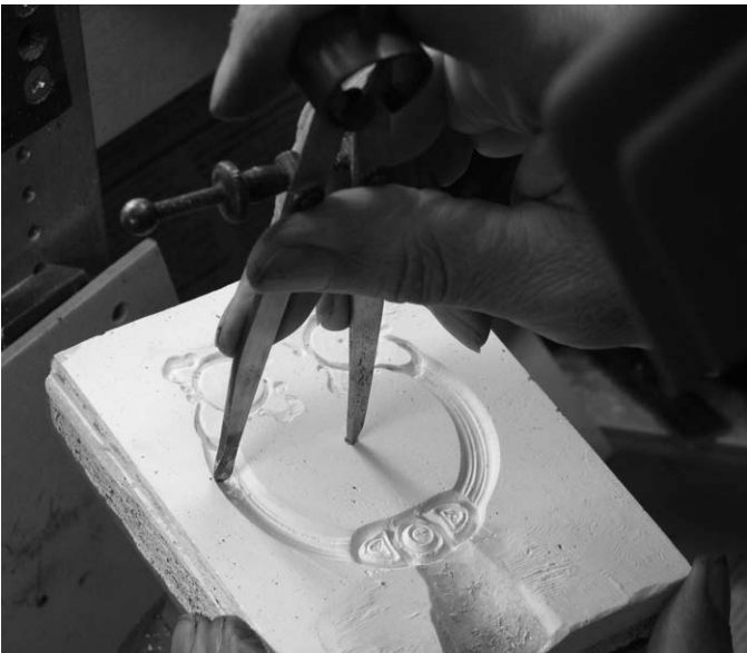
8. The duplicate moulds usually need some re-carving to clean up irregularities from the clay impressions. A compass with the moving leg sharpened into a gouge is used to trace the arc of the loop of the brooch in the same way that the master mould was originally carved.
