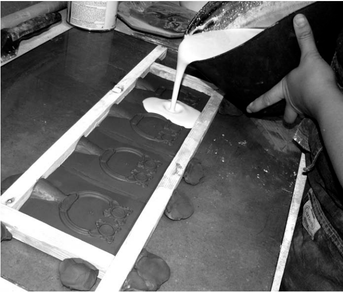
7. Plaster is poured directly on wet clay impressions of the master mould to make duplicate plaster moulds. Each mould used to cast metal can only be used once.
