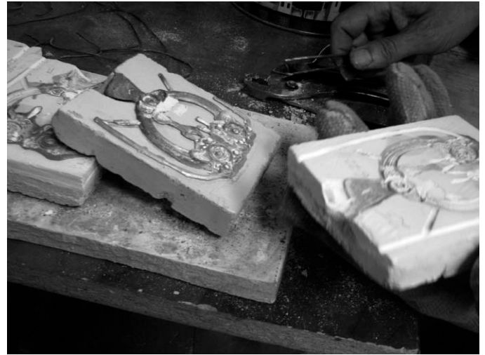
12. Mould opened after casting with molten silver. The button of silver at the funnel and the risers will be cut off along with the fins of metal that flowed between the two halves of the mould.
