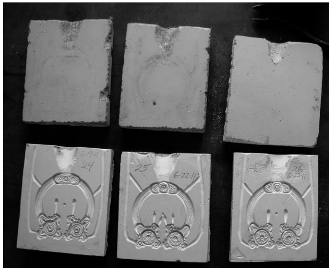
11. Moulds with backs for brooches 24, 25 & 26. Each mould has a funnel entering the brooch at the cartouche as well as riser channels to allow air to escape ahead of the molten silver.
