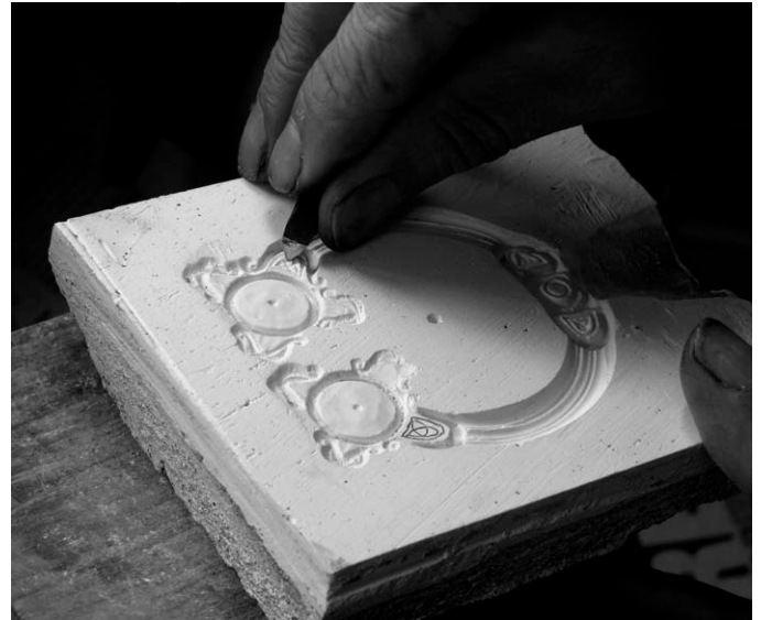
9. Interlace chip carving is carved in the negative using a "V" graver. This mould will be used to copy brooch 26. The chip-carving in each brooch is different.
