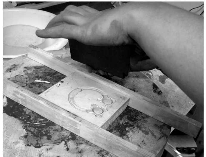
6. Multiple potter's clay impressions are used to copy the master mould.
