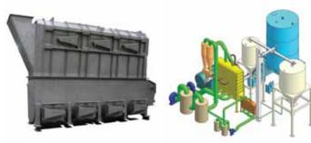
Schwing Bioset's fluid bed dryer offers a thermally efficient means of producing dust-free Class 'A' biosolids. Automated to allow unattended operation, the Fluid Bed dryer operates under completely inert conditions and, unlike other technologies, it does not require any recycle of already dried biosolids.
