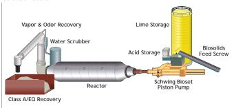
As the Bioset process is totally enclosed within the reactor the process operates odor free. The reactor discharge provides the only location for gases to escape and they are easily collected and scrubbed utilizing a small water scrubber. The resulting final product has an odor that is similar to wet-concrete.
