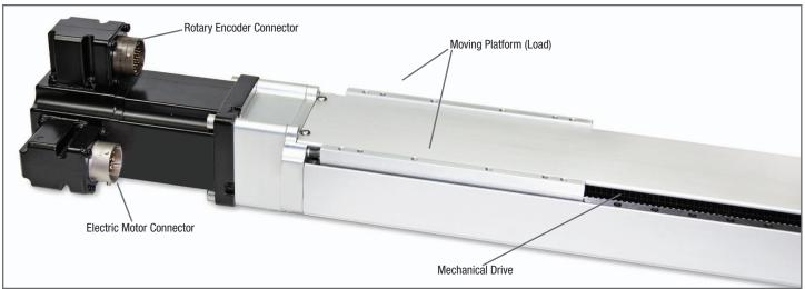
The indirect load monitoring system showin in this application includes an electric motor directly coupled to a rotary shaft encoder, which acts as the load position sensor. In this setup, although the rotary encoder accurately indicates the drive motor's shaft position, the true standard of measurement is not the rotary encoder, but the drive system itself.
