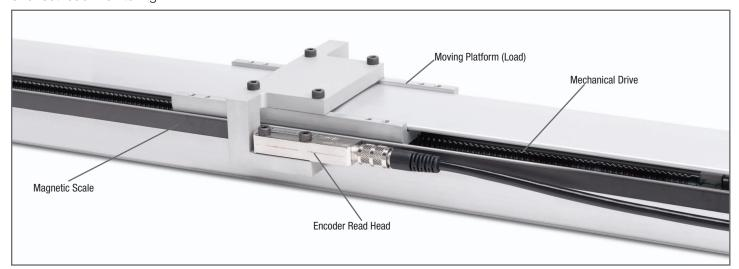
A system architecture where the linear encoder is located along the controlled motion axis is an example of direct load monitoring. By simply relocating the position data collection point from the motor shaft to the linear motion axis itself, drive—system stack—up errors can largely be ignored. In this arrangement, motor shaft revolutions do not need to be directly proportional to load position, because of the linear encoder is now directly reporting load position.
