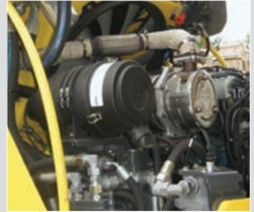
Tier 4 Final Kubota diesel engine
