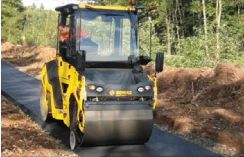
The optional cab and edge roller features will increase machine versatility for all weather conditions
