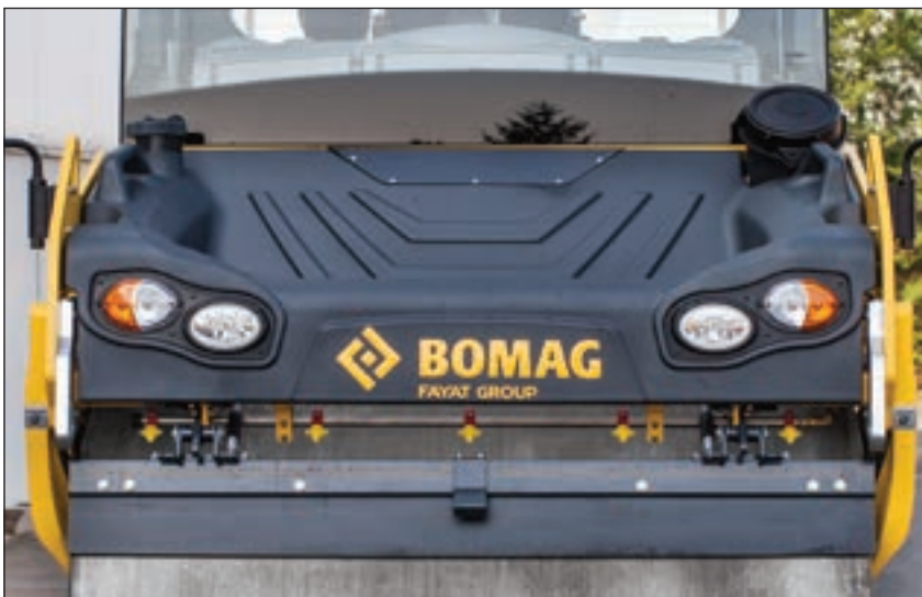
Triple filtered water spray system with backup reserve pump and easy clean nozzles
