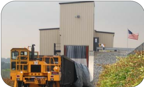
MHF Track Mobile positioning lined gondola railcars into North Bergen Transload Facility.
