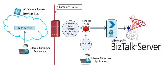
Sentinet Nodes can also be deployed in the hybrid deployment scenarios, where some Nodes are deployed on-premises while others are in the cloud. Both consumer and service applications can be fully decoupled from Windows Azure Service Bus specific APIs and security configurations.
