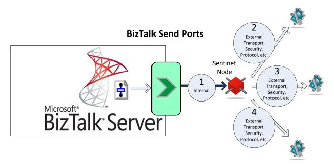
Sentinet software platform supports the industry standard and all Microsoft-specific communication and security protocols, and can mediate between interoperable and Microsoft-specific message exchanges.
