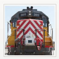
ROVER<sup>™</sup> installed on a SD-40. MU cable and air lines hooked up. Approximately 30 minutes to install.
