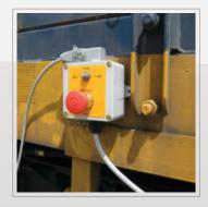
Locomotive mounted emergency stops located on both sides.
