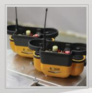
Ergonomic OCU units. Two assigned per locomotive for pitch and catch operations.
