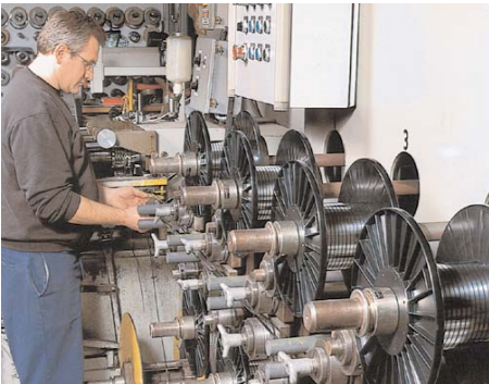
This multihead slitter cuts several narrow widths at a time and recoils the strip on oscillate wound spoos.
