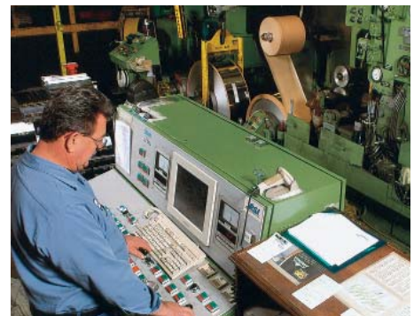
This high speed Z-mill is equipped with automatic gauge control to instantly adjust the roll bite and maintain the desired gauge and close tolerances.
