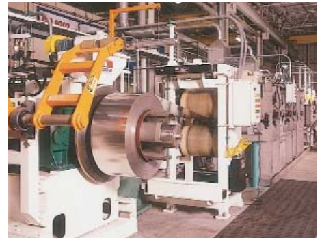
This high pressure hot water jet cleaning system is used for applications requiring ultra clean surfaces.
