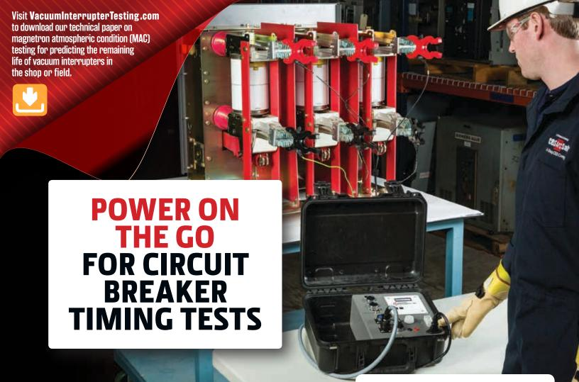
CBT-1201 includes heavy-duty circuit breaker timing test set, power supply, and switching controls all in one unit.
