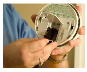
Smoke alarms are powered by battery or they are hardwired into the home's electrical system. If the smoke alarm is powered by battery, it runs on either a disposable 9-volt battery or a non-replaceable 10-year lithium ("long-life") battery. A backup battery is usually present on hardwired alarms and may need to be replaced.
