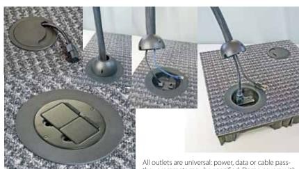
thru grommets may be specified. Dome covers with flexible conduit provide an uncluttered harness to the furniture. These replace the standard, hinged covers. RJ45 data connections are standard. Specify custom connectors as required.
