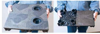
Interchangeable carpet tiles self-adhere to a set of four pedestals. This allows flex, so they float on the floor without laser leveling. Universal outlet ports for power, data, AV or pass-thru may be located in any of the pedestals. Pedestals are 3" high, providing a generous cable way capacity. Weight capacity tested to 40,000 lbs for each pedestal. 20 US tons.
