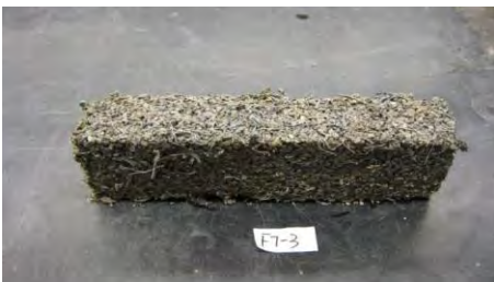
2 ¼” fiber at 7.5 lb/cy at 300 cycles retained almost complete integrity
