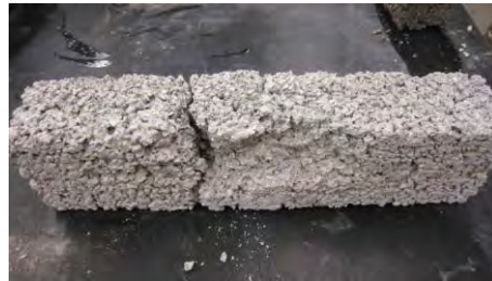
1 ½” fiber at 2.5 lb/cy failed at 133 cycles in single-crack mode
