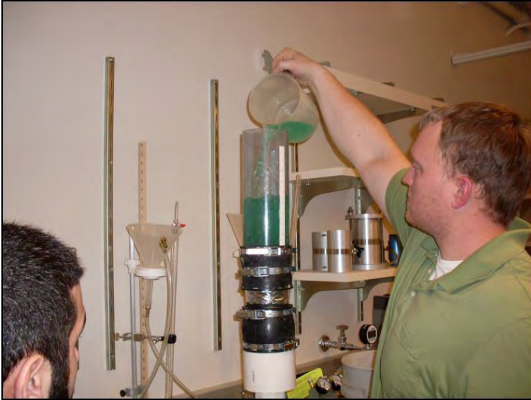
Permeameter Testing (Green Water Shown for Contrast)
