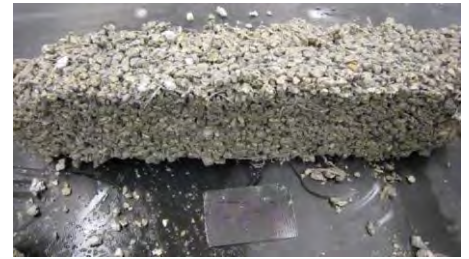
1 ½” fiber at 5.0 lb/cy failed at 188 cycles yet retained integrity
