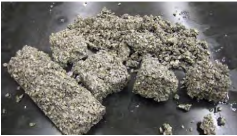
Control mixture failed at 187 cycles with complete loss of integrity
