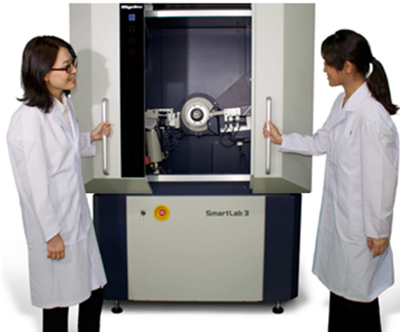
The Rigaku SmartLab 3 Intelligent X-ray diffraction system
