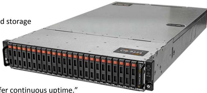
The CiB-9224 utilizes energy efficient DDR4 memory, integrated 10Gb Ethernet ports and can scale by adding external JBODs through Avago® DataBolt™ SAS expander technology. This unique architecture eliminates additional hardware costs, minimizes footprint requirements, and simplifies cabling and installation, enabling optimal uptime high availability (HA) and maximizes storage performance for I/O-intensive applications, cloud datacenters and virtualized server environments.
