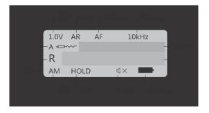
**PRIMARY DISPLAY:** The Primary Display is located in the middle of the screen and uses the largest font. It shows the dominant impedance parameter reading typically with 5 digits displayed.
