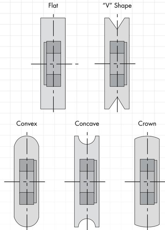
Any profile can be custom designed to last the life of the application. Or for a drop-in replacement for existing sliding door designs, a standard roller can be paired with a custom shaft.
