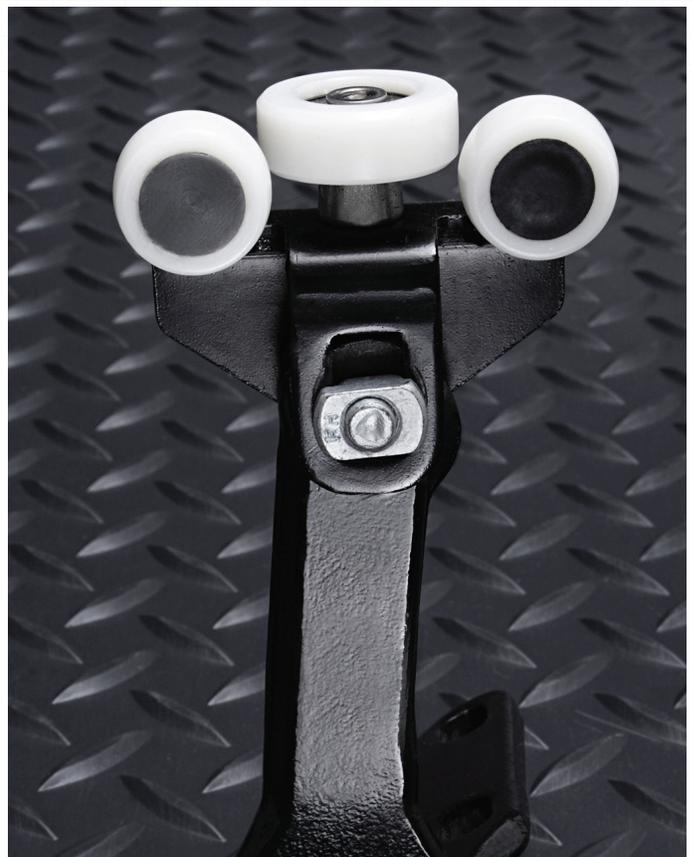
Vehicle doors, particularly those on vans for passenger and commercial use, have to withstand millions of trouble-free openings. Hybrid rollers have proven to be a successful selling feature.
