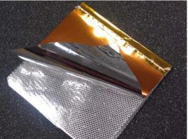
each component of the spacecraft, then sewn together and secured with polyimide tapes. The resulting MLI blankets both absorb and reflect radiant energy and provide protection against impact from micrometeoroids.
