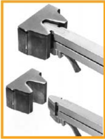
“Gap-by-Gap” gear hardening principle and typical inductor designs
