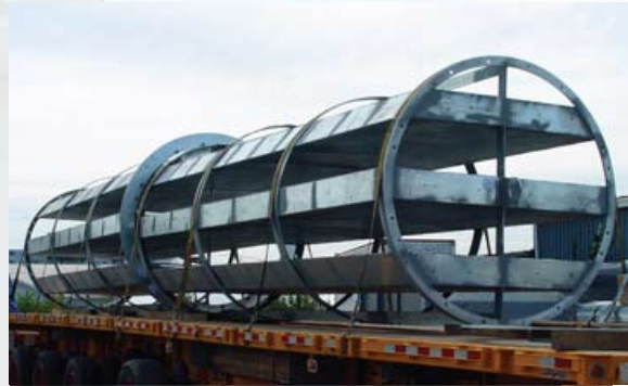
Circular Stack Inlet Silencer
