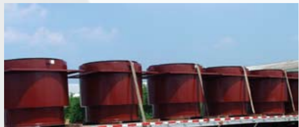
Building Exhaust Stack Silencer
