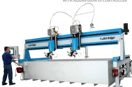
Jet Edge's EDGE X-5° 5-axis waterjet system cuts complex taper-free and 3D parts from virtually any material. Featuring Jet Edge's innovative Permalign EDGE technology, the EDGE X-5 dramatically increases your waterjet cutting capabilities by allowing you to produce chamfers, weld bevels and sophisticated 3D parts such as impeller blades - all with a taper-free finish.
