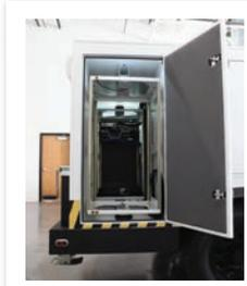
Electronics bay includes air ride system anti-vibration stabilizers for the 42 rack units of space. Separate breakers on each rack power circuit provides diverse power management. The 'closed air' electronics bay has dedicated A/C and Heat keeping vital equipment in optimal operating temperature range.
