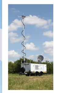
pCom XL is designed to be deployed in the most remote conditions and left running for weeks. The tower provides ideal Cellular, Radio, Video, or other device which can be managed via the satellite network.
