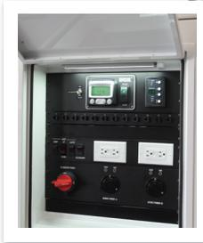
External I/O panel allows for control of the pCom electronics, pneumatics, scene lighting, air conditioning and power generation from a single secure panel. Cable management allows for 'runs' into other buildings from the I/O patch panel.
