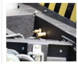
pCom has a brass grounding rod attachment locations and pneumatic air "Quick Connects" for use with air tools.
