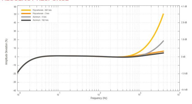
This data was generated with an aluminum unit (gray) bolted with 100 in-oz torque, and a polycarbonate unit (orange) mounted with double sided tape.
