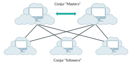
• **Cloud-friendly network architecture:** Conjur only needs to be reachable on two ports: 443 (https) and 636 (ldaps). By distributing followers wherever they are needed, there is no need to set up complex network security and routing configurations in order to allow the servers to reach Conjur; followers should be placed where needed (e.g. in the private subnets), and connect to the master for replication on the fly
