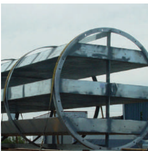
Circular Stack Inlet Silencer
