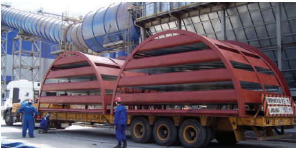
Stack Silencer for South American Power Plant
