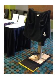
for the user then when the user is ready to put it on, she backs up to the device and is able to position her arms in the sleeves. By pressing down on a foot pedal the clothing is brought up to her shoulders and she is then able to complete the donning task.
