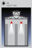
When ambient light goes below the preset illumination level. or down to 0%, lamps switch on automatically
