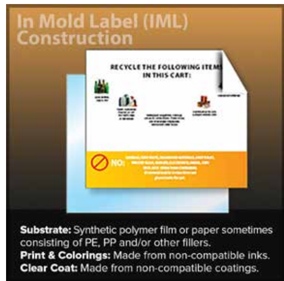
FIGURE 1. In Mold Label Construction
