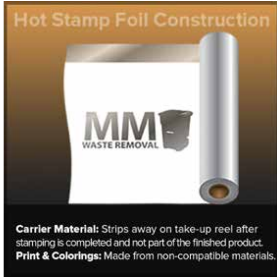
FIGURE 2. Hot Stamp Foil Construction
