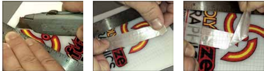
FIGURE 7. ASTM D3359-09 Crosshatch Tape Test
