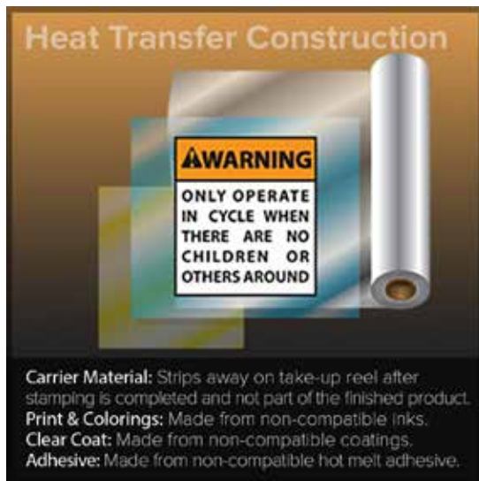
FIGURE 3. Heat Transfer Construction
