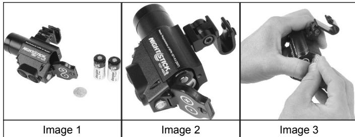
To install the included CR-123 Lithium Batteries in the 4650, begin by unscrewing the screw on the battery compartment door. (Image 1)
