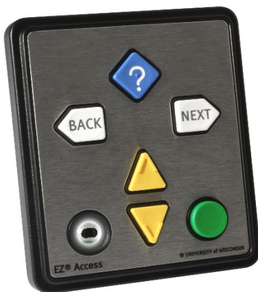
Figure 3 The audio enabled EZ-Access keypad
