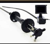
Bore Measurement Head Mounted to Borescope
