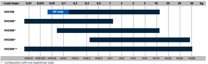
\*\* configuration with one low and one high load loadcell per scale
