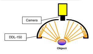
The dome shape gives this product a particular advantage in uniformity when illuminating and reading OCR codes on reflective or round surfaces.
