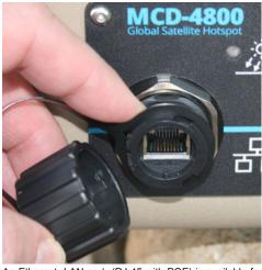
An Ethernet LAN port (RJ-45 with POE) is available for a hard wire Internet connections. Normally it is capped sealed when not in use
