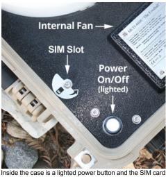
tray. The internal fan helps keep electronics cool if tempretures rise. It is recommended to open the case to help vent excess heat buildup in hot weather.
