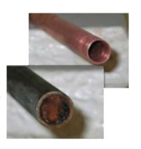
So-Blu heat-transfer fluid contains special rust inhibitors that protect your pipes against corrosion and buildup. What's more, So-Blu doesn't break down during extreme heat and also acts as an anti-freeze, protecting your pipes and collectors from bursting when the weather turns cold.
