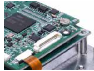
12 position, 1.25 mm picoblade connector shown with protective cover plate removed
