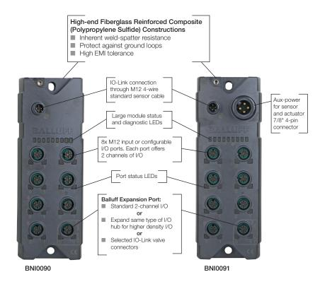
All Weldblock family I/O hubs have the Balluff Expansion port available as standard. The expansion port can be used as a standard I/O (or input only in case of input hub), or expanded with same type of the I/O hub one time only to provide higher density I/O or connected to one of the following IO-Link valve connectors for actuating valves:
